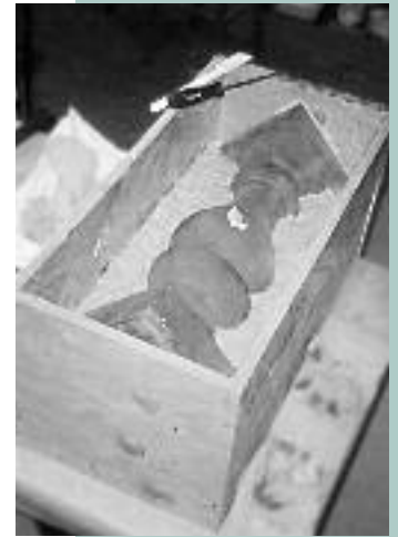
The original baluster is placed in sand, liquid is poured, and a mold is made.
